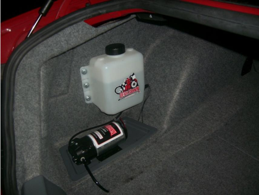
Figure 2: Pump placement
